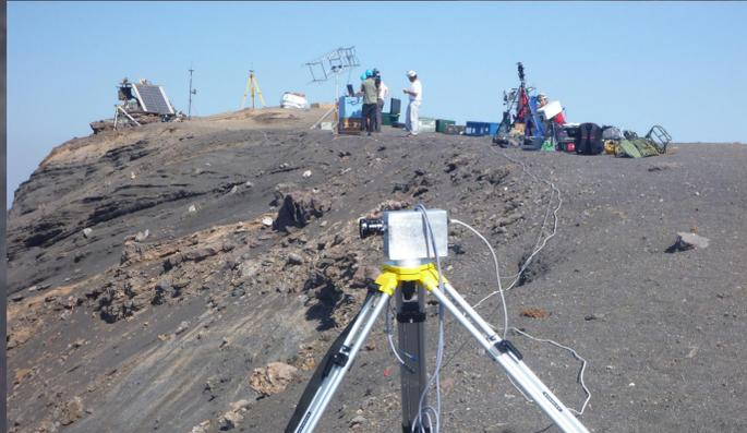
**One laser disdrometer** (Parsivel OTT) This was deployed to test its potential application to collect information on the sizes of ash particles, along with ash collectors and direct sampling.
