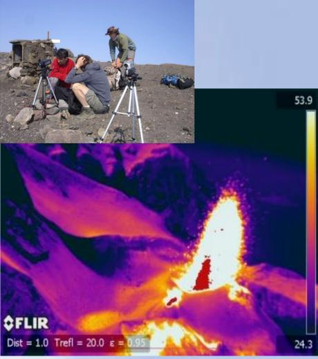
**Two thermal infrared cameras** (FLIR Systems cameras, 8-14 microns) One camera was deployed to track, at 200 Hz, hot gas and particle velocities, particle size distributions and mass fluxes across a narrow window immediately above the vent. A second camera imaged, at 30 Hz, plume ascent and dispersion.
