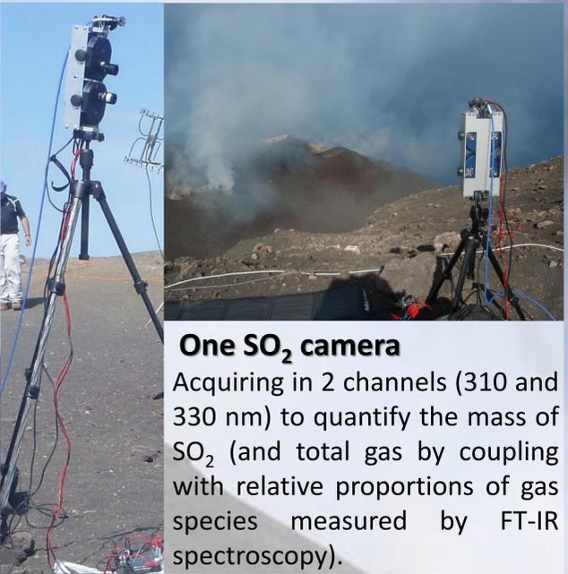
**One SO<sub>2</sub> camera** Acquiring in 2 channels (310 and 330 nm) to quantify the mass of SO<sub>2</sub> (and total gas by coupling with relative proportions of gas species measured by FT-IR spectroscopy).
