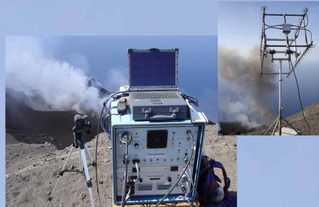
**One Doppler radar** (VOLDORAD 2/OPGC, 23.5 cm wavelength) VOLDORAD2 was deployed to quantify the mass and ejection velocities of ballistics. Using these data, we will be able to simulate the reflected energy at VOLDORAD's wavelength to compare with measured radar echoes and with results of a ballistic model to infer source parameters including pyroclast initial velocity, mass, and mass flux.
